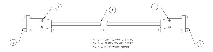
PIN 2 - TXD PIN 3 - RXD PIN 5 - GND
